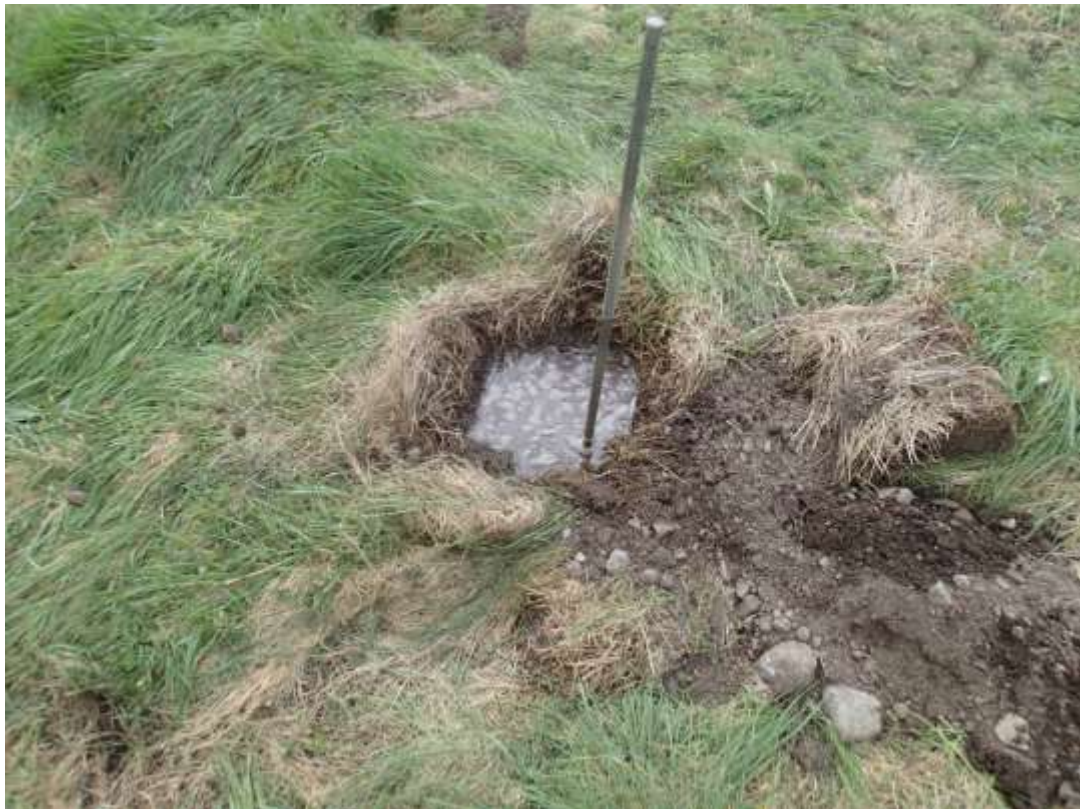
Plate 8: Water falling on morning of Tuesday 12 th May 2015 in ‘P’ test hole number 1.
