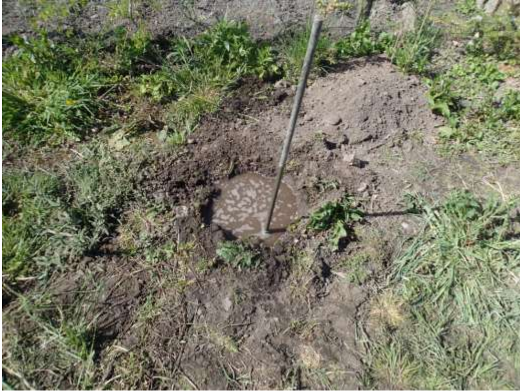
Plate 11: Water falling on morning of Tuesday 12 th May 2015 in ‘P’ test hole number 4.
