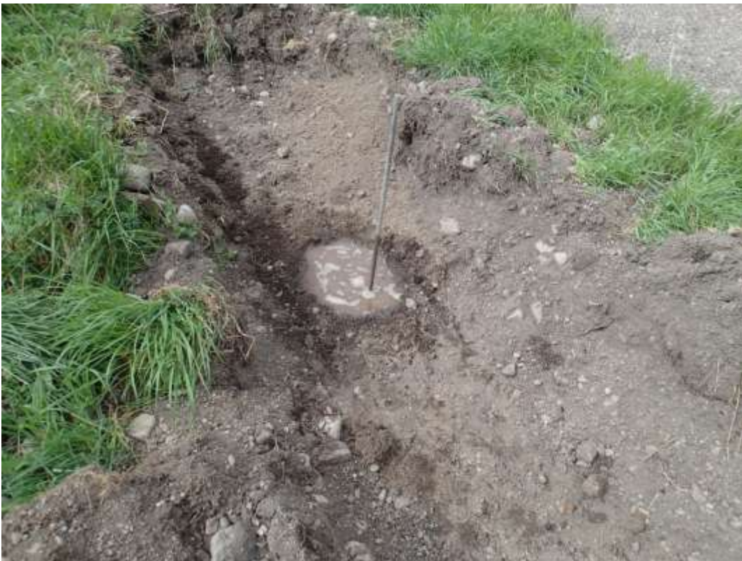
Plate 6: Water falling on morning of Tuesday 12 th May 2015 in ‘T’ test hole number 3.
