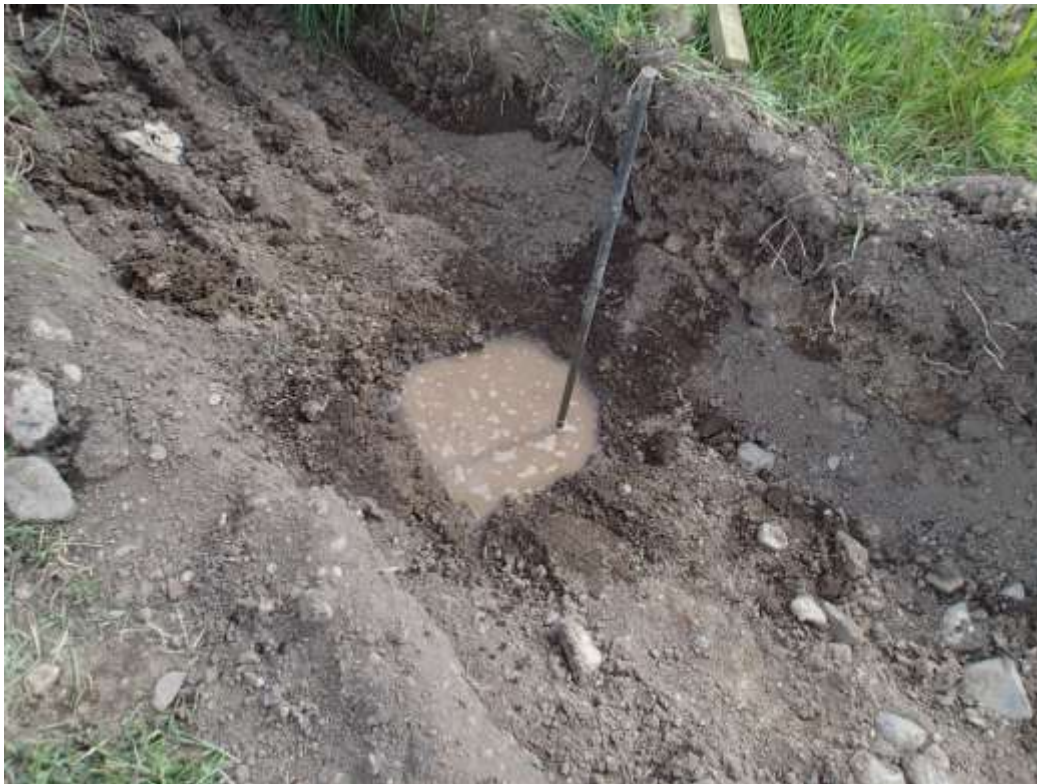
Plate 4: Water falling on morning of Tuesday 12 th May 2015 in 'T' test hole number 1.
