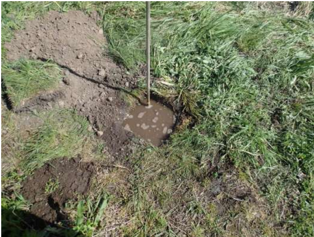
Plate 10: Water falling on morning of Tuesday 12 th May 2015 in ‘P’ test hole number 3.
