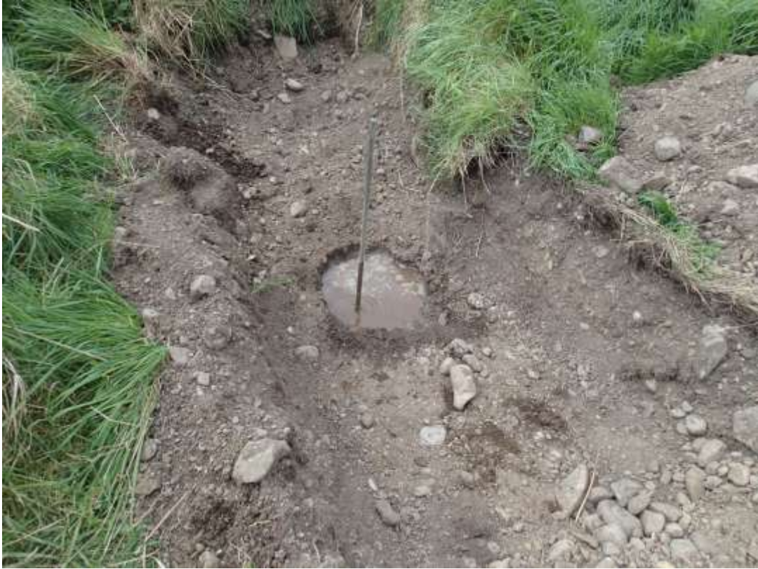
Plate 7: Water falling on morning of Tuesday 12 th May 2015 in ‘T’ test hole number 4.
