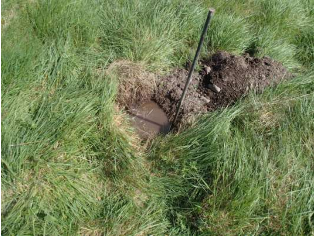
Plate 9: Water falling on morning of Tuesday 12 th May 2015 in ‘P’ test hole number 2.
